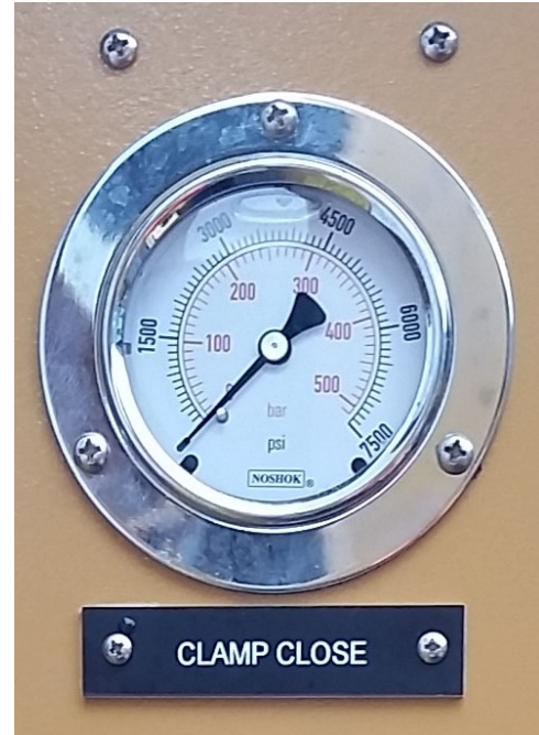
Power unit clamp CLOSE dial as seen beside the power unit control panel. Pressure measured in psi and bar.
