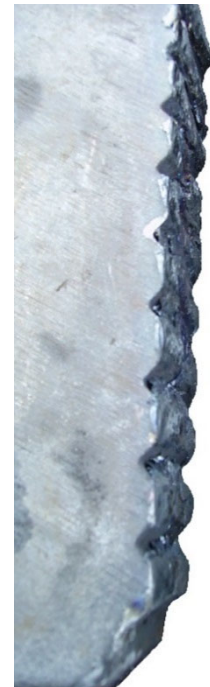
Unevenly worn jaws in need of prompt replacement.
