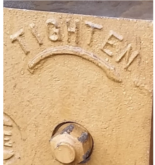
Caisson TIGHTEN label appears on one side of the clamp above the wedge screws.
